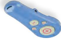
The LRC 1/8" Jack Input: By connecting an external device to this port, left and right mouse clicks can be activated from the external device instead of from LRC keypad.
