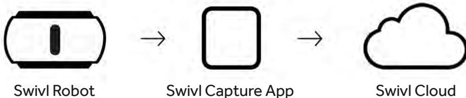
Swivl works by receiving an infrared signal from a small remote (marker) you hold or wear. Set your mobile device into the dock and Swivl rotates and tilts to follow you as you move around the classroom. The marker's built-in microphone captures wireless audio while your mobile device\* uses our app to record video, which you can then upload to our private hosting service.
