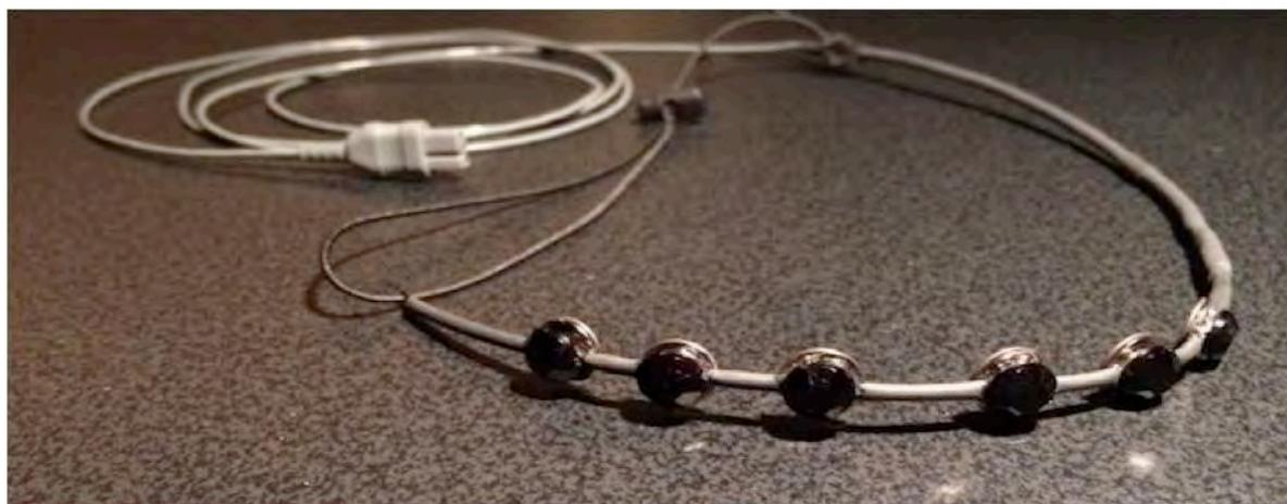
Below the electrode-skin connection is the scalp, forehead muscles, skull and a container filled with cerebrospinal fluid in which floats the brain. All are electrically conductive. An electrical signal from brain neural impulse activity travels through the conductive layers to the surface of the skin.
