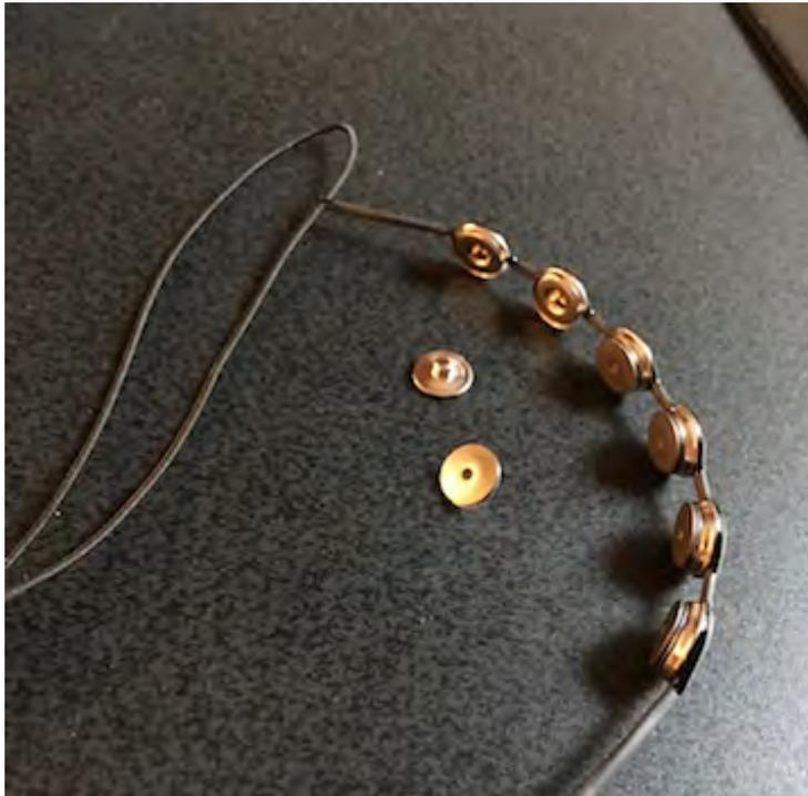
It is best to clean the headband and sensors with a soap and water wipe. Antibacterial soap can be used. Alcohol should not be used as soaking the black epoxy in alcohol can degrade the epoxy coating.
